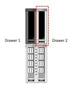
Installed the re-timer card to the upper-right bracket for drawer 2 (2:H2)
