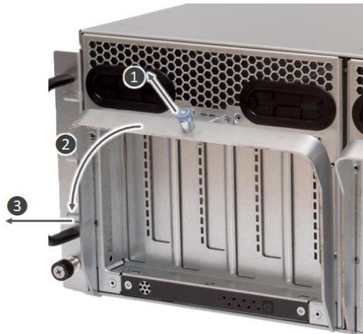
To fully remove the drawer from Falcon 4016, please push the safety latch on the bottom right hand side of the drawer. This latch becomes visible once the drawer has been withdrawn to the halfway point, see the image below.
